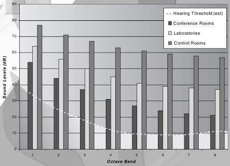
Decibels are a logarithmic ratio: For instance an increase in the sound pressure level of 3 decibels represents twice the sound intensity. And an increase of 10 decibels represents ten times the sound intensity.
