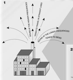
1: Sound at the higher frequencies tends to travel in straight lines and is more effectively contained by noise barriers. Low frequency energy tends to diffract at the barrier boundaries.
