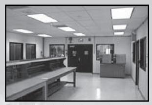
Test enclosure for hazardous machinery device evaluation. Controls and monitors to regulate the test environment as well as both wet and dry fire suppression are installed.
